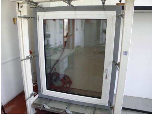
Fig. 1 Test specimen on test rig window closed
